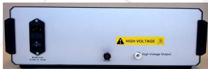
Rear panel views of Techimp HVDC Generator.
